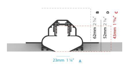
A: OPENING WIDTH B: RECESS DEPTH C: OPENING DEPTH D: PROFILE HEIGHT E: WIDTH INCLUDING MOUNTING BRACKETS
